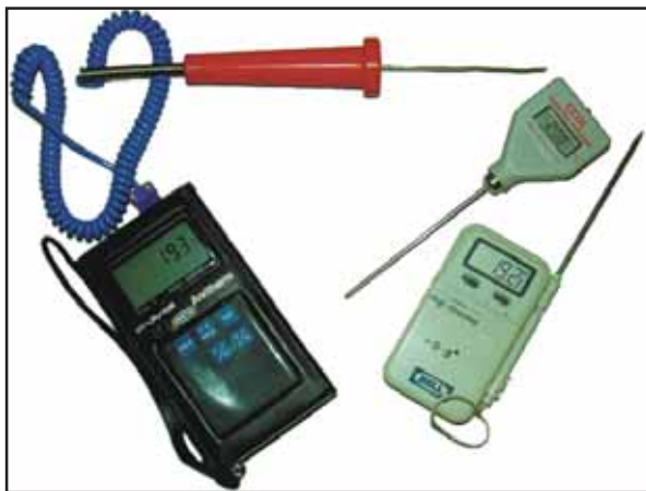
Probe thermometers are the only way to properly measure vegetable core temperature.
